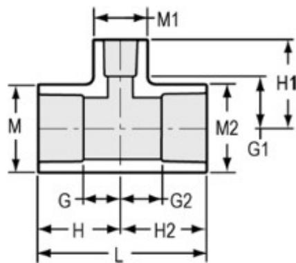
**Connection** Socket x Socket x Socket
