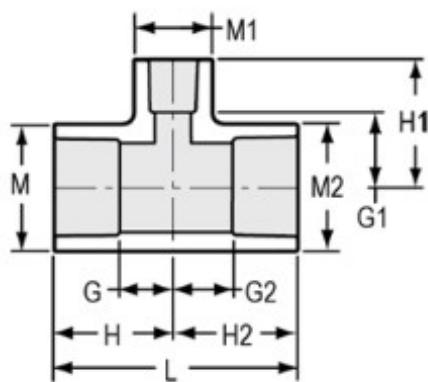
Connection: Socket x Socket x Socket
