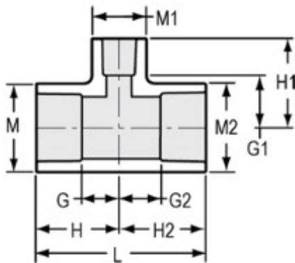
Connection: Socket x Socket x Socket
