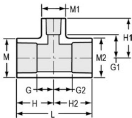
Connection    Socket x Socket x Socket
