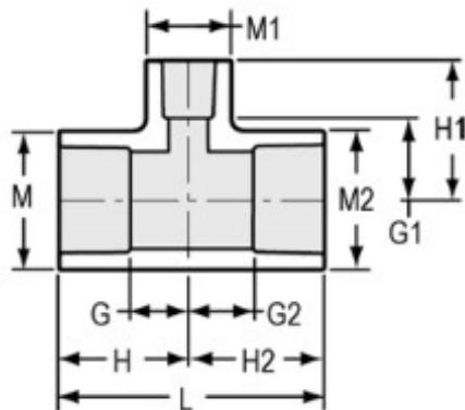
Connection: Socket x Socket x Socket
