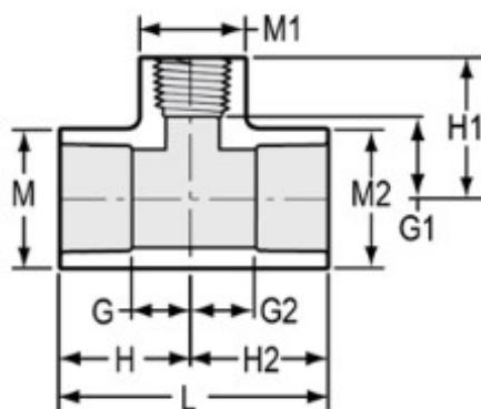
**Connection**    Socket x Socket x Fipt**Type**    Reduction**M1** = 1- 5/8**M2** = 2- 1/4**L** = 4-1/4**M** = 2- 1/4**G1** = 1-11/32**G2** = 13/16**H** = 2-1/8**H1** = 2-1/4**H2** = 2-1/8**G** = 13/16
