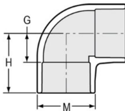
**G** = 9/16**H** = 1- 1/2**M** = 1-5/16**Connection**   **Socket x Socket****Angle**   90°**Type**   Standard
