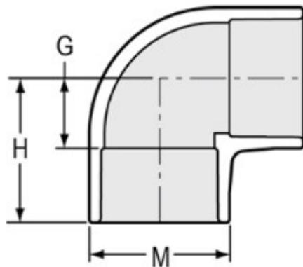
**G** = 3-9/16**H** = 6-9/16**M** = 7-9/32**Connection:** Socket x Socket**Angle:** 90°**Type:** Standard
