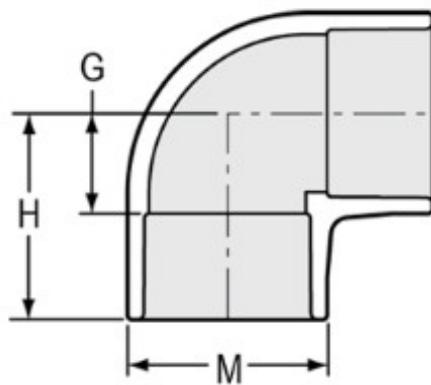
**G =** 5-27/32**H =** 10-27/32**M =** 11-19/32**Connection**    **Socket x Socket****Angle**    **90°****Type**    **Standard**
