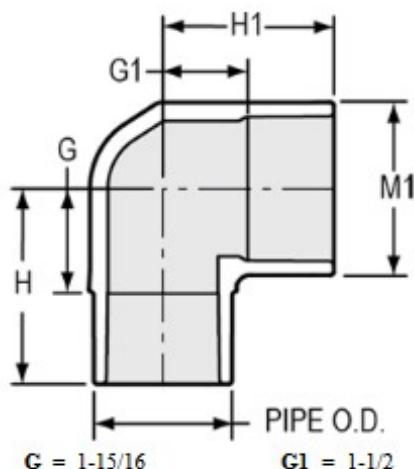
**G** = 1-15/16**G1** = 1-1/2**H** = 3-11/16**H1** = 3-1/4**M1** = 3-11/32**Connection** Spigot x Socket**Angle** 90°**Type** Standard
