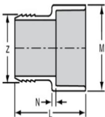
**L** = 3**M** = 2-13/16**N** = 3/16**Z** = 2-3/32**Connection** Insert x Socket**Type** Standard
